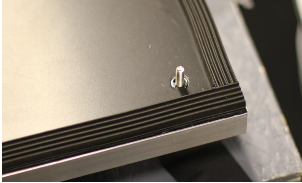
Figure 7. The seal selected for the enclosure door.
