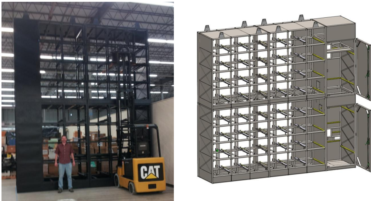
Figure 3. Left: the first VIRUS enclosure being stacked at Texas A&M University; right: a model of the enclosure with the added annex.
